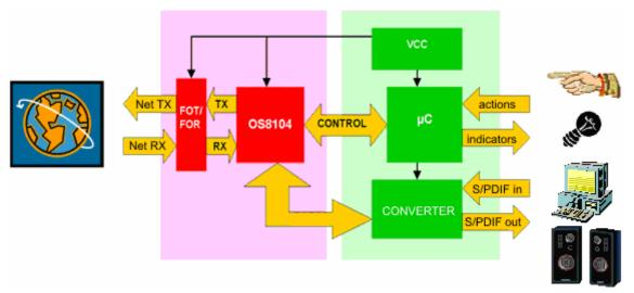
Fig. 1 a) Block diagram of the basic node with the Physical layer board (PLB) on the left and the application firmware board (AFB) on the right, showing their external connections and functions.
